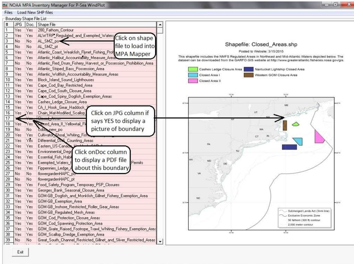
To make a new boundary the shape file has to be converted for use with WindPlot. To load a boundary shape file, click the FILES menu for a list of all shape file as shown above (if they were loaded from the CD). If nothing appears in the list, then try reloading the Importer program.
